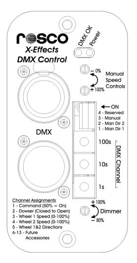
By turning DIP switch #3 ON, the module is placed into manual mode.
