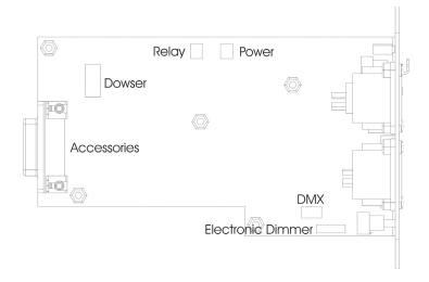
For the most part, connectors can be matched up to headers on the PCB. The only exception is the relay and power headers, which are identical. The relay cable uses two blue wires while the power cable uses a red/black combination.
