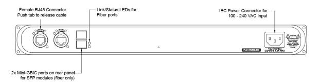
Models 6750 and 6750-P require the user to provide an SFP (small-form pluggable) fiber adaptor to allow connection of the mini-GBIC ports to fiber optic networks. See Appendix 1 for recommendations on SFP adaptor selection.
