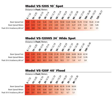
All peak UV-A irradiance measurements taken at beam center using UVX Digital Radiometer and a calibrated 365nm sensor
