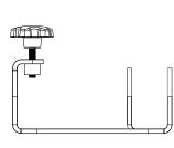
Kit: PMA Bracket 8mm Knob Assembly 4-M8 x 30mm Bolts 4-M8 Washers
