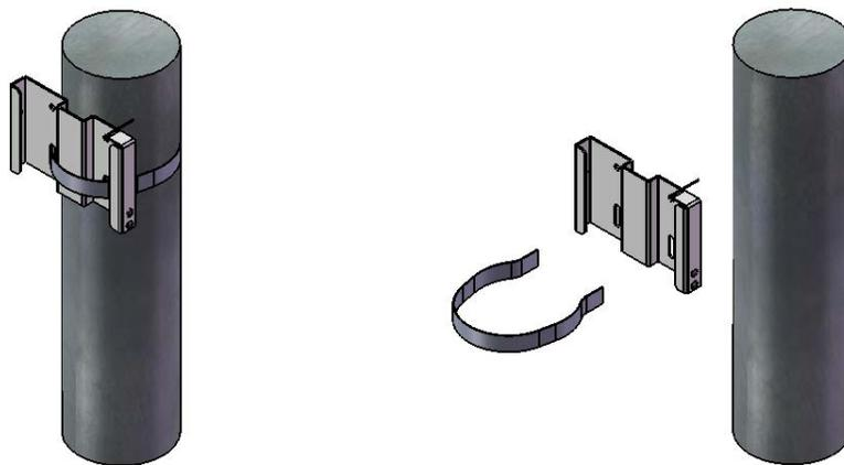
Slide the mating Mounting Bracket (attached to the Unit) into the Mounting Bracket Base until the locking clip engages, and install the retaining Screw.
