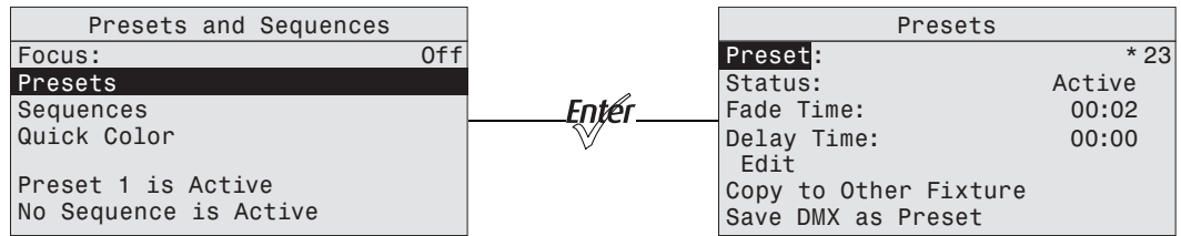
Figure-4.16 Selecting Presets on the Presets and Sequences Menu
