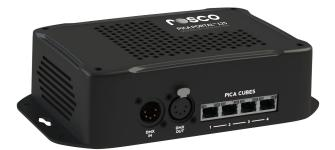
To connect Pica Cubes to the Pica Portal, simply plug the Pica Portal into AC power and then connect it to a DMX control source using a 5-pin DMX cable. From there, connect up to four Pica Cubes to the output ports on the Pica Portal using standard CAT5 Ethernet cables. The Pica Portal is convection cooled, has built in electrical safety features and features integral mounting points for ease of installation.
