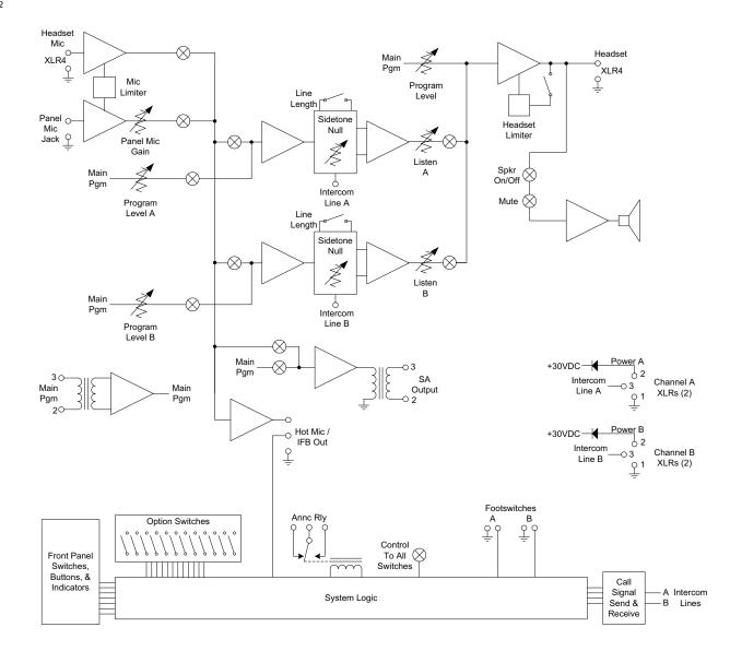
Figure 3-18: Audio Block Diagram for the RM-702
