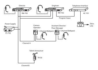
Figure 2-10: Typical ENG/EFP Truck Installation
