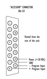
Figure 2-13: Connecting Program Sources
