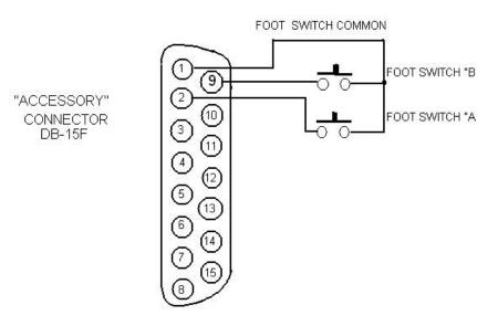
Figure 2-17: Connection of External Talk Switches
