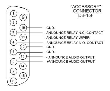
Figure 2-16: Connections for Announce Audio and Relay Outputs
