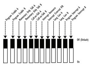
Figure 2-7: DIP switches
