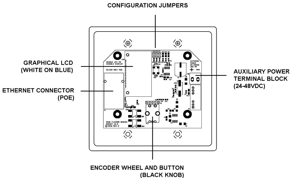
Using the LCD, encoder, and jumpers, an installer can commission the PRE10E-A. Initial commissioning consists of setting the following configuration options:
