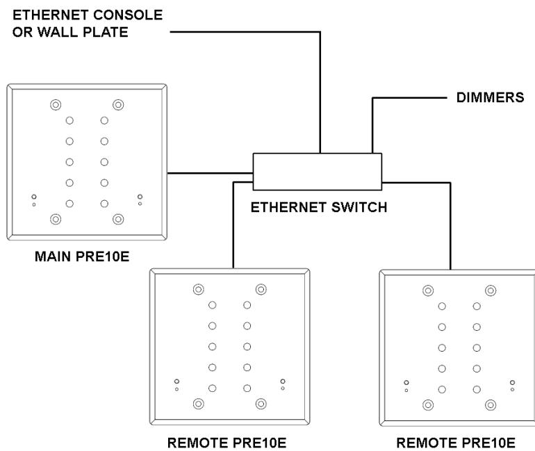
Data transport between each sACN capable device takes place using standard Ethernet hardware that supports multicast traffic. The above diagrams utilize a single Ethernet switch for simplicity. Any network hardware constituting a properly configured LAN may replace the Ethernet Switch blocks above.
