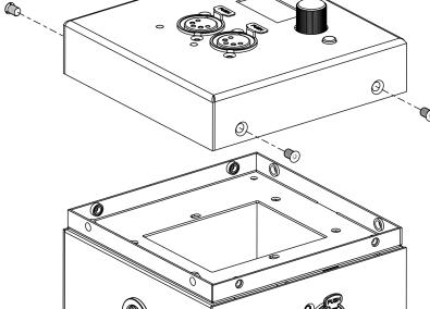
Once a qualified technician/electrician has reconnected the control surface panel with the power and data connectors, the control surface panel can then be mounted and secured to the base assembly with (4) torx-screws.
