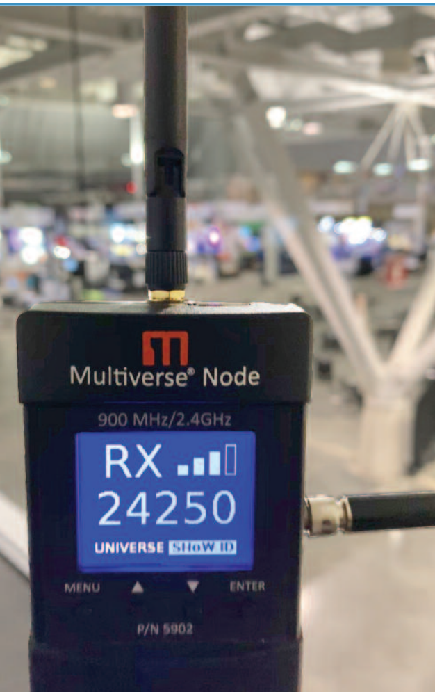
At a distance of approximately 500' or more, I had good signal strength using the 2.4GHz band in a crowded space.
