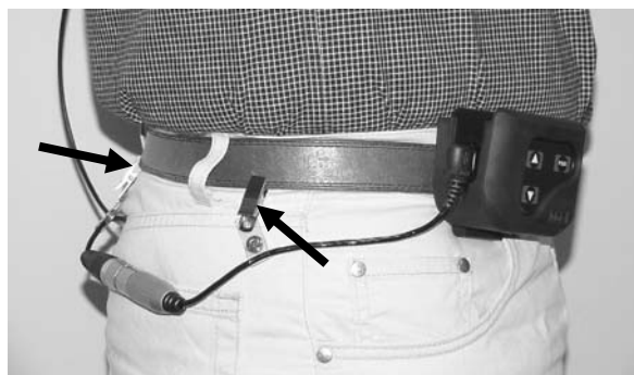
Figure 2. Clip cables to belt or clothing
