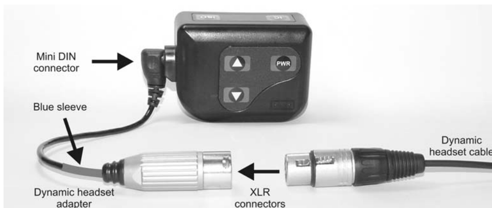
Figure 1. Connect mini-DIN connector to Beltpac and XLR adapter to headset
