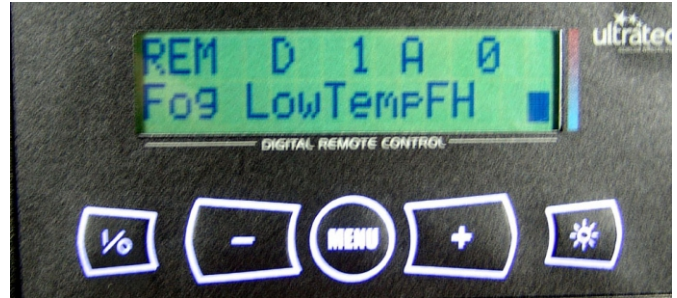
Note error from trying to turn on machine that is not yet hot enough.
