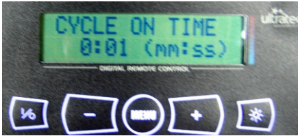
Menu screens for timer on/off function with remote control only. DMX control ignores these setting.
