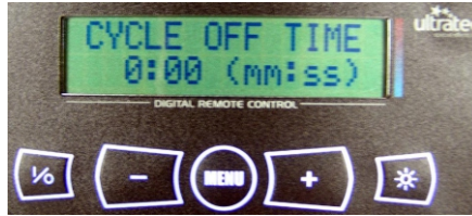
Menu screens for timer on/off function with remote control only. DMX control ignores these setting.
