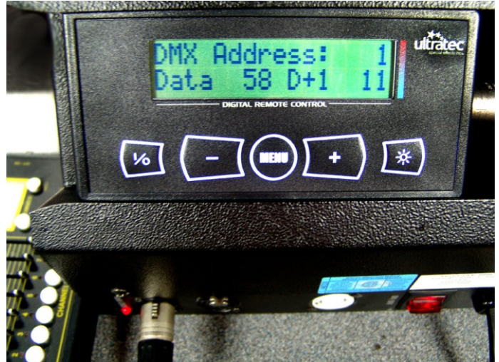
DMX address selection screen. This shows DMX set to channel 1. Channel 1 data is 58 (0-255) channel 2 is 11.
