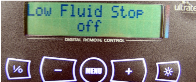
If set the Fog output stops when fluid gets low (F indicator on main screen).
