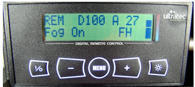
Machine on with remote. Not fully heated (see temp bar and H is on) so requesting 100% but getting 27%.
