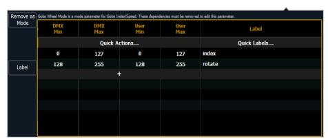
After patching the new fixture, you will be able to check your modes in the encoder display and ML controls. There are now buttons for the modes, and for index, the degree symbol is displayed with the user value.
