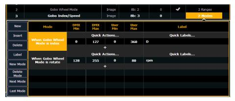
Assign the DMX and user values. The range values were used for the DMX values. For index, the user values were set to 0-360 degrees. The quick label for degree unit was used so the degree symbol will display in the encoder display. For rotate, the user values were to 0-80 rpms.
