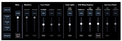
This menu allows you to adjust the brightness and contrast settings for your console's face panel, as well as any internal monitors, supported external monitors, fader wings, and task lights. All sliders have a range from 0% (dimmest) to 100% (brightest).
