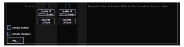
When enabled, a launching window will display on start-up. If a network connection is not made, you will have the option to **Start Anyway**}, **Start Offline**}, or to **Cancel**.
