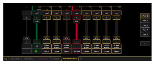
The virtual fader module has a configuration menu, which is accessed by first selecting the module tab and then double clicking on the tab to open the menu. With the virtual fader module selected, you can also select the gear icon, which is located by the tabs, to open the configuration menu.
