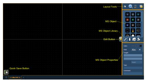
The main area of the magic sheet will display a grid to aid with layout. The editing tools will be displayed on the right side of the magic sheet. The editing tool window is divided up into three areas: layout tools, the MS Object Library, which is made up of four tabs that contain the MS Objects, and the MS Object Properties.
