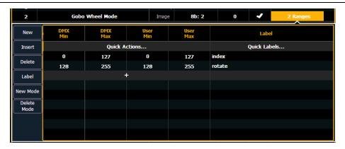
Back in the fixture editor, assign a parameter as gobo index/speed. Click in the range column to open the range editor. Press **{New Mode}** to create two modes.
