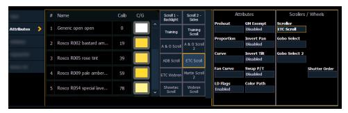
The picker displays on the left half of the CIA when you select the specific attribute (**Scroller**), **{Color Wheel}**, **{Gobo Wheel}**, or **{Effect Wheels}**). The picker displayed is specific to the selected attribute (the scroll picker will display when **{Scroller}** is pressed, the color wheel picker will display when **{Color Wheel}** is pressed, and so on).
