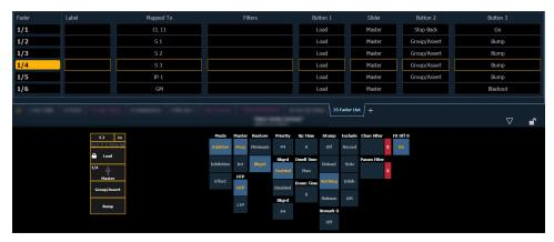
You can also make changes to a fader's configuration while in the fader list display by clicking on a column. A virtual fader will be displayed. Click on the appropriate area of the fader to access the configuration options. Selection can be done by clicking in the column or from the command line.
