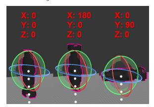
The above left example shows the default orientation of 0/0/0, or pointing straight down. The center shows a rotation of 180° about the X axis, pointing the fixture straight up. The final example shows a rotation of 90° about the Y axis, pointing the fixture to the side.
