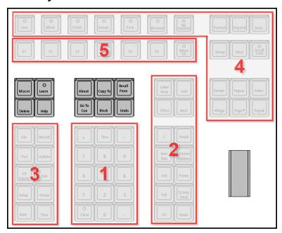
Backlit hardkeys are provided on the face panel. The brightness level for those keys can be adjusted in the *Brightness Settings* (on page 182).
