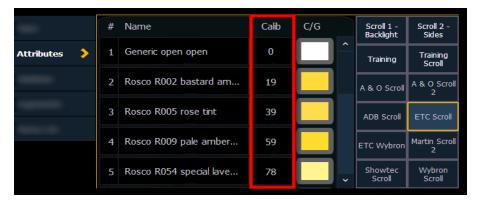
The displayed calibration information is the DMX level that puts the frame into its center position. Information in the calibration column can be manually edited by clicking on it and typing in a new DMX level.
