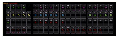
When the summary view has been collapsed to show only intensity data, you may include focus, color, or beam data in the summary view by holding down the **[Params]** key and pressing any parameter category key. This displays all categories again. On Element 2, you will need to use **[Data]**.
