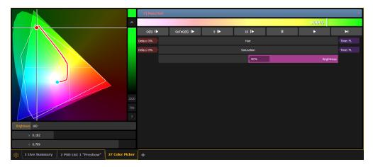
Changes can be stored in the destination cue as absolute data by using **[Update]** or **[Record]**. When there's a change to the color path information, a red c will display next to the channel number and the color path's name will display in red in the color path display. When that data has been saved, a blue c will display. The color path's name will also display in blue in the color path display.
