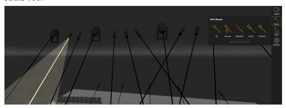
Stick Beams draws a line from the fixture to wherever the beam lands. Stick Beams do not require intensity and can be used to focus a fixture that is not currently outputting.
