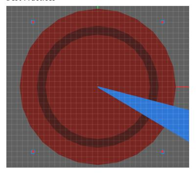
There are many ways to select FPE Point positions. The preferred method is to use at least 4 points close to the bounds of your space, as in the example above. Larger angles between points reduces the possibility of redundant information being used in the calculation. It may help to think of the points as outlining the base of a 3D shape that should cover as much of your space as possible.
