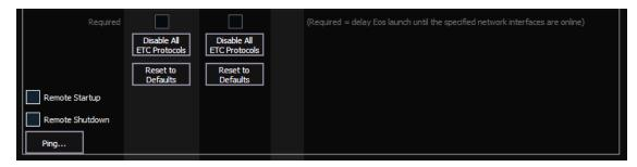
Using this button will disable all currently-enabled output, interface, DHCP, and SNTP protocols for the selected network port.
