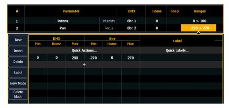
If a parameter has only one range, the values for that range will display in the range column. If that parameter has multiple ranges, the number of ranges will be displayed. If a range is used in a mode, the range will not be in bold.
