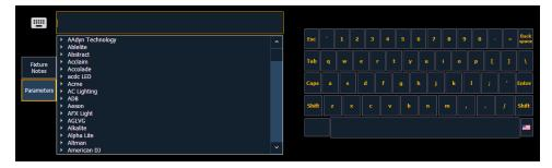
In the search window, press {Parameters} to view a parameter list for a fixture, or press {Fixture Notes} to see any notes that exist for it. You can also view this information in the Fixture Editor.
