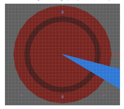
A better (but still problematic) configuration is pictured above. Since one of the points is in a line between two others, the data from that point is redundant and cannot be used to calculate the fixtures' positions.
