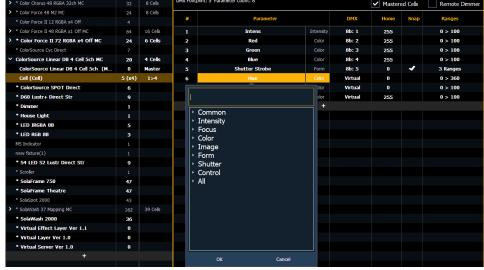
To change specific cell data such as DMX offset, you will need to use **{Edit Multicell}**. With a multicell fixture or a master cell selected in the fixture editor, press **{Edit Multicell}**. In the Edit Multicell window, you can edit cell numbers, DMX offset, and mastered cells for each cell.
