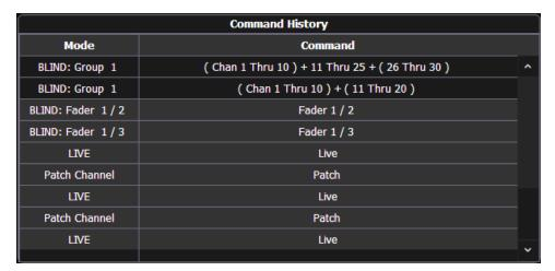
You may use the page arrow keys or a mouse to select multiple commands. When **[Enter]** is pressed, an advisory is posted. When **[Enter]** is pressed again, all highlighted commands will be undone and subsequently removed from the command history. When removing more than one command, a confirmation is required.
