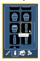
From the second tab, fixture symbols can be placed on a magic sheet. The symbols can be tied to a channel number. Information about that channel can be displayed with the symbol, such as intensity, FCB data, and error indicators. See *MS Object Properties* (on page 426) for more information on the customizing options available.
