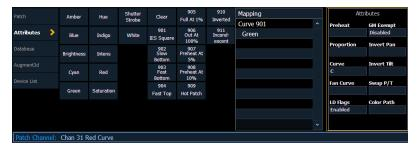
Eos provides ten pre-programmed, commonly used curves. They can be edited or copied to a new curve location. When a pre-established curve is deleted, it will return to its original state.
