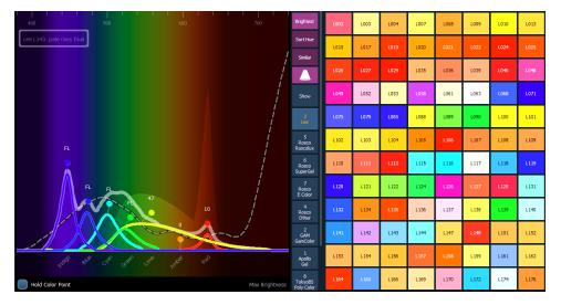
**{Hold Color Point}** allows you to adjust individual emitters and the other emitters will automatically adjust to hold the color selected. This can only be used with fixtures that have more than three color parameters.
