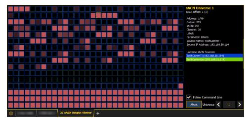
The left side of the viewer is the universe grid. It displays 512 address cells. Cells outlined in a color are currently patched addresses. Each patched cell contains an address number and output value. Unpatched cells are black and only have an address level.
