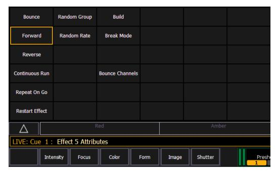
**{Restart Effect}** is an attribute that can only be accessed from this display. When enabled, **{Restart Effect}** will cause an effect to restart whenever the cue is fired. This attribute is applied to the cue that the effect is stored in and not in the effect itself.
