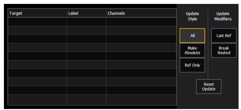
The dialogue box also provides you with a listing (by record target) of what channels/parameters will be impacted by the update instruction. If the channel contains a reference in the cue, it is indicated. Channels that have been manually added to the stage output, but are not overrides of an active cue will update to the selected cue list.
