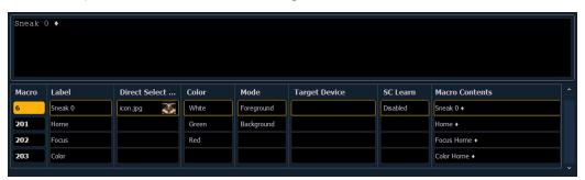
While in the macro editor display, any numeric entry on the command line is assumed to be a macro number. If the macro number entered already exists and [Enter] is pressed, the macro list will page to the selected macro and the macro content detail section will display all of the contents of the selected macro. If the macro number entered does not exist in the list and [Enter] is pressed, an empty macro will be created with the specified macro number.
