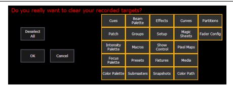
From the **{Clear Targets}** screen you can select which record targets you wish to clear. The buttons at the center of the CIA represent all of the record targets that you can choose to clear. By default all components are selected (gray) and will be cleared. To withhold any targets from being cleared, simply deselect them in the CIA by clicking the respective button. To deselect all of the targets, click the **{Deselect All}** button.
