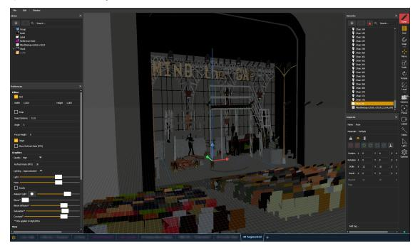
Surrounding the central workspace are primary windows to assist in fixture and object manipulation: the Library, Materials, Preferences, Hierarchy, and Inspector. These windows can be freely dragged, rearranged, re-sized, and closed.
