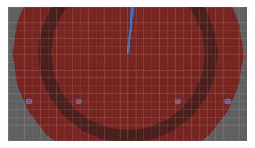
One example of a poor configuration is shown above, with all FPE points in a line. The two center points are redundant, as they are part of the line from the two end points. Additionally, there is no coverage of the stage space possible with all points arranged in a line.
