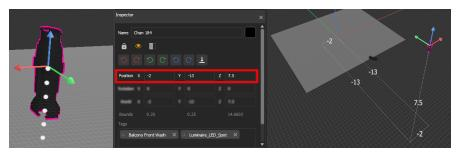
In the above example, the fixture patched to Channel 184 is -2 meters offset on the X axis, -13 meters offset on the Y axis, and 7.5 meters offset on the Z axis.
