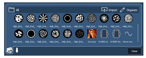
Any targets that can be applied to a direct select (other than channels and scenes) can be assigned an icon, which can be configured to appear on the direct select button in Direct Selects (Tab 4) or Custom Direct Selects (Tab 39). See *Custom Direct Selects* (on page 91) and *Configuring Direct Selects* (on page 89).
