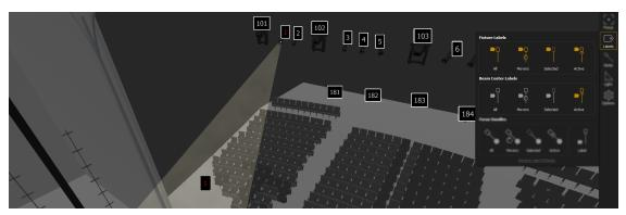
Fixture Labels display the channel number of the fixture. This can be useful in identifying which fixture is creating a particular beam of light.
