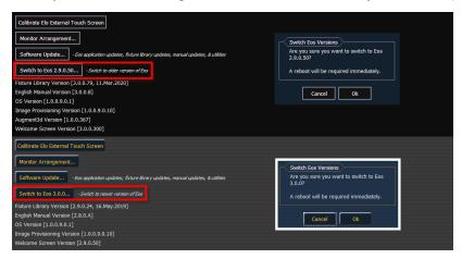
Use the "Switch to" button to alternate between versions. A restart will be required before any changes can take effect.
