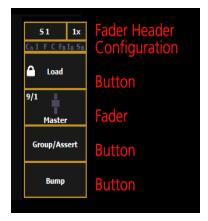
Each fader is color coded based on its assigned target type. Grandmasters and inhibitive submasters are in red, additive submasters are yellow, playback faders display in green, and presets, palettes, global effects, and manual time masters are orange.
