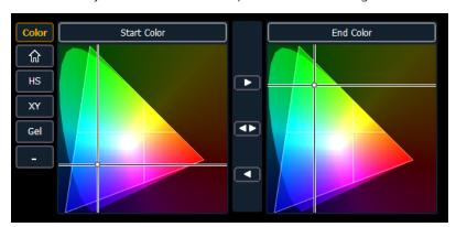
Using the buttons located between the two color pickers, you can also copy the start color to the end color, swap the start color and the end color, or copy the end color to the start color.
