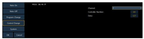
Control Change commands were designed to represent specific actions on MIDI devices, like pedals actuations and effects. For example, the Damper Pedal on a keyboard is often represented by controller number 64 (hex 40). Similar to MIDI Note commands, the MIDI data that is expected to be received is shown in the CIA and changes as you select event parameters. When finished configuring the control change event, press **{OK}** to store the event. Otherwise, press **{Cancel}** to undo the changes.
