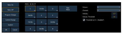
Note On and Note Off commands simulate activating (on) and releasing (off) a musical note. The MIDI data that is expected to be received is shown above the Note selection area, with 'N' shown where any valid number will be considered a match. This display will change as configuration options are selected. When finished configuring a Note On or Note Off event, press {OK} to store the event. Otherwise, press {Cancel} to undo the changes.
