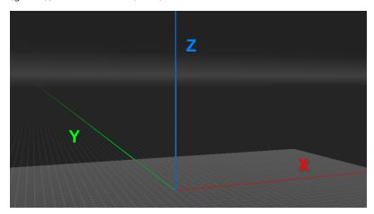
The point at the intersection of these axes (0,0,0) is the origin. This virtual point in Augment3d must correspond to a real point in your space, ideally on the floor. This could be in the center of your stage, in a corner, or any convenient point.
