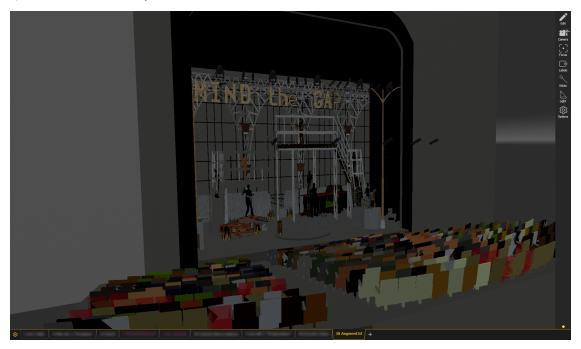
Collectively, the Augment3d virtual environment is referred to as the model. All fixtures and objects must be part of the model in order to be configured.
