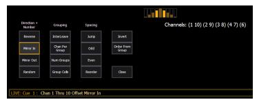
The following options are available as extensions of **{Offset}**. Options can be used together. These extensions can be used to create *Subgroups* (on page 221). To close the Offset display, press **{Close}**.
