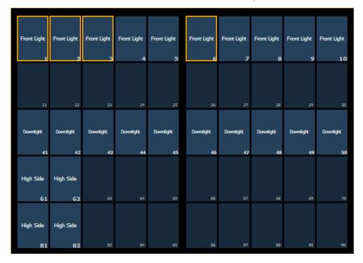
Channel selection from the direct selects is an additive process. When a channel is selected, it is added to the current selection set. To select only one channel and deselect all others, double-press the channel touchbutton.
