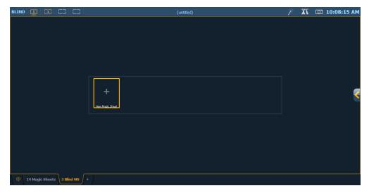
After you have created a magic sheet, you can recall a specific magic sheet, by pressing [Displays] {Magic Sheet} [#] [Enter] or you can navigate to Displays> Record Targets>Magic Sheet and press [Select] to open the magic sheet list (see Magic Sheet List (below)).
