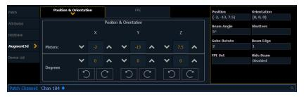
Under the Augment3d section in Patch, fixtures have fields for XYZ Position and Orientation. If the fixture is nested, this data is relative to the parent. World Position and Orientation are absolute, relative to the scene overall. If nested, an arrow indicator will apear next to the position and orientation fields. For more information about nesting, see *Nesting Objects*.
