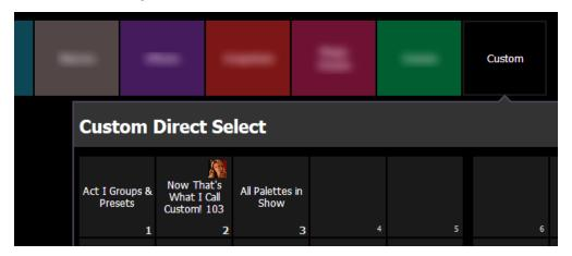
Once a custom direct select list is open, selecting an empty button will display a popup of the *Target Selection Menu (2) (on page 91)*, allowing you to quickly assign a target or range of targets.
