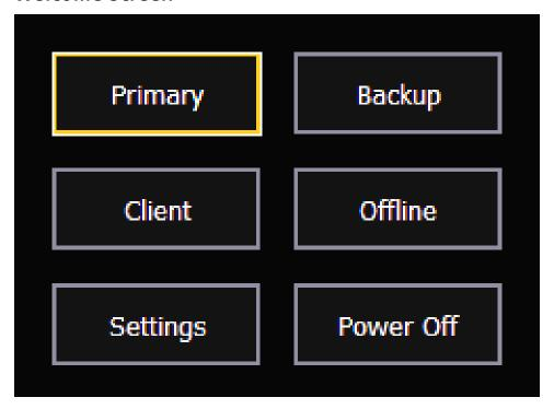
This is the starting screen of the utility. From here you can choose to boot the console in one of several different modes, change various settings, or shutdown the console.
