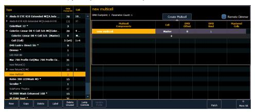
2. Press **{+}** to add cells. This will open a fixture list display. Only fixtures added to your fixture list will be here.
