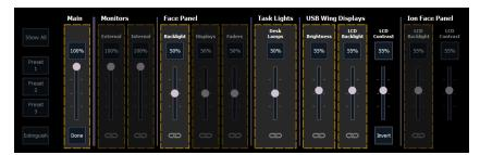
When **{Link to Main}** is selected, any linked brightness sliders are outlined in yellow. Unlinked sliders are not outlined, and display a broken link icon underneath. Click the icon to toggle between linked and unlinked. LCD Contrast sliders cannot be linked.
