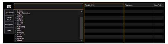
Select the Lightwright device and the match from the Eos column. Multiple Lightwright devices can be selected at a time. Then click **{Link Devices}**. The link will appear in the Mapping column. To unlink a device, select it from the Mapping column, and then press **{Unlink Device}**.
