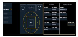
In this display, you can invert the **{Shutter Order}** or rotate the order using the arrow buttons. After you have created the order needed, press **{Apply}** for your changes to take effect.
