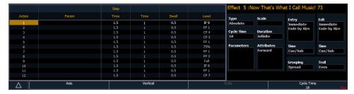
In the above image, actions 1 through 7 indicate referenced values in the "Level" column (palettes or presets), though these values can be absolute data as well.
