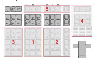
Backlit hardkeys are provided on the face panel. The brightness level for those keys can be adjusted in the *Brightness Settings* (on page 182).
