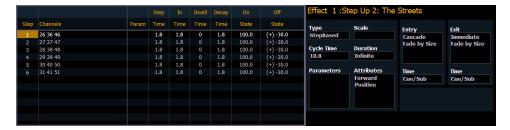
If an effect step is on the command line or indicated in the blue text to the left of the command line, entering a number on the command line will default to selecting a step for the current selected effect.
