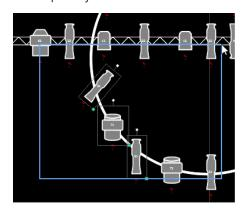
Selecting from right to left will open the green crossing selection box. This selects any object that either crosses the boundary line of the box or is completely inside of it. This can be done with a single touch or using a mouse.
