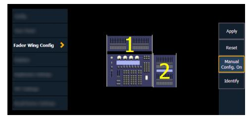
Click and drag the wings to match your physical layout. Click **{Apply}** to save the changes. Clicking **{Reset}** will restore to the last saved configuration. Clicking **{Manual Config. On}** will turn off manual configuration and will require a restart of the application before the console will automatically configure the wings.
