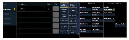
You can label the new wheel by pressing [Label] and typing the desired label on the virtual keyboard and pressing {Enter}.
