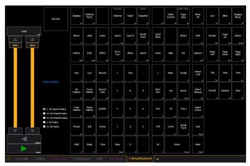
The virtual keyboard displays the alphanumeric keyboard shortcut for that hardkey in the lower right hard corner.
