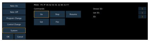
System commands allow you to specify specific MIDI Show Control messages that can be received and interpreted by the console. While any MIDI Show Control command that matches the configured Device ID will be executed normally, this type of event setup allows you to respond to messages sent to different device IDs, or take additional actions based on a show control command.
