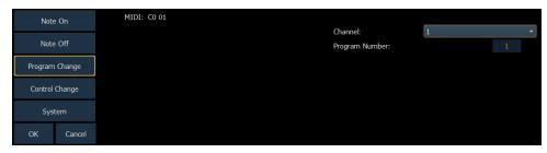
Program Change commands typically represent a change in the MIDI voice or instrument type that should be used for a particular MIDI channel. Similar to MIDI Note commands, the MIDI data that is expected to be received is shown in the CIA and changes as you select event parameters. When finished configuring the program change event, press **{OK}** to store the event. Otherwise, press **{Cancel}** to undo the changes.
