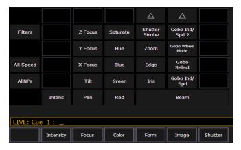
Within the CIA, in the upper left corner, notice the **{All NPs}** button. When pressed, this collects all non-intensity parameters for further editing.
