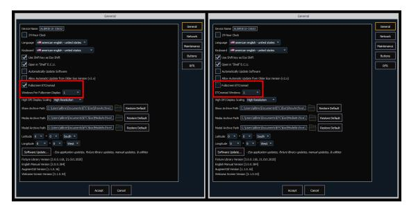
When the "Fullscreen ETCnomad" box is checked, ETCnomad will automatically launch fullscreen, on all connected monitors of your computer. Select "1" in the "Windows Per Fullscreen Display" dropdown to show a single fullscreen ETCnomad display on each monitor, or "2" to subdivide each fullscreen display into 2 ETCnomad windows.
