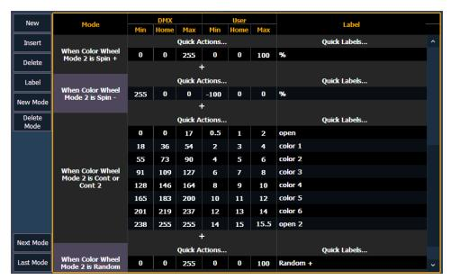
When viewing a fixture profile, the parameters that have modes will display the number of modes in the ranges column.
