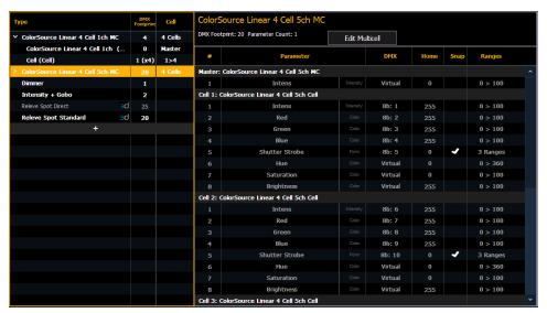
On the right, you can see the full personality of the selected multicell fixture. If you have the whole fixture selected, you will be able to see all of the parameters for each cell and the master but changes cannot be made here.
