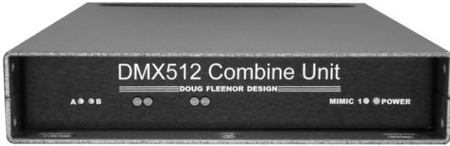
The DMX512 Combine unit solves the problem of combining multiple DMX input signals into a single DMX output signal. The most common configuration of the unit allows two consoles to control a single set of dimmers in a *highest takes precedence* or *pile on* mode. Examples of where this might be necessary include booth console/stage manager's console, primary console/backup
