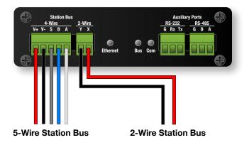
A maximum of fifty (50) 5-Wire stations can be connected to a single CueStation Hub. The maximum distance from the Hub to the farthest 5-Wire Station is 4000 feet (1220m).
