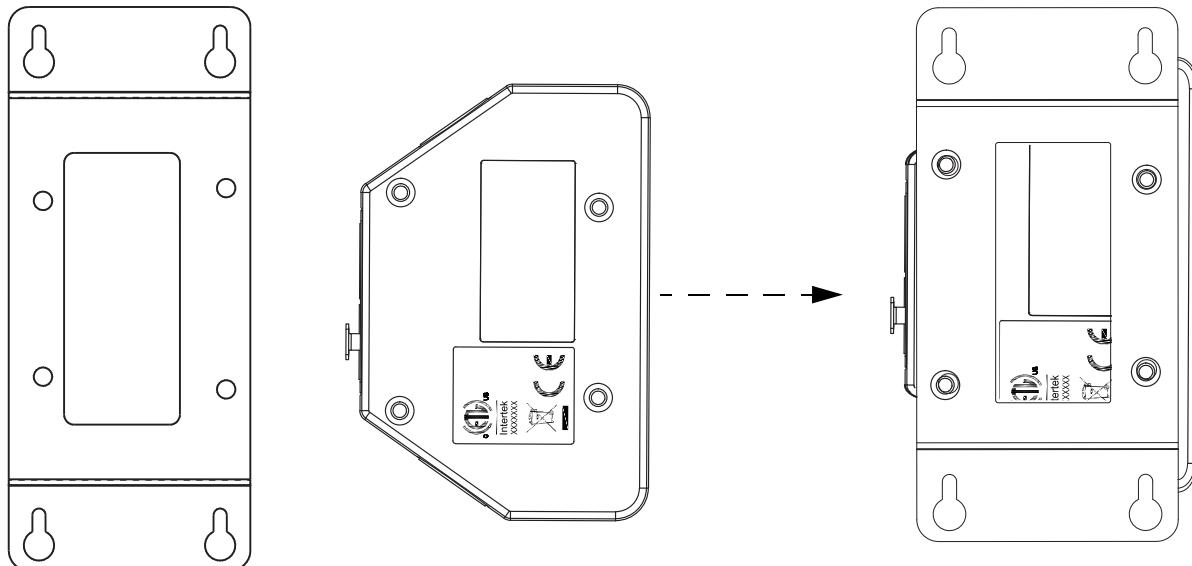
Step 2: Using a Philips head screwdriver, attach the bracket to the relay with the included M5 screws.
