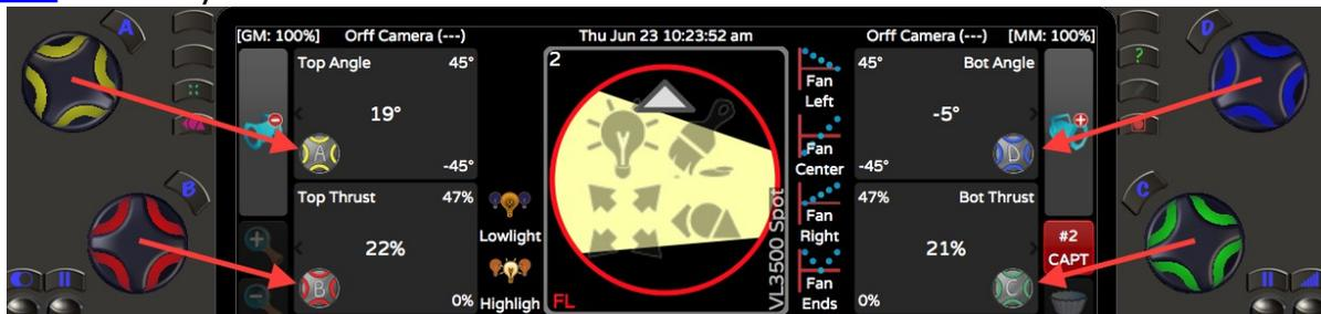
Wheels are used to directly adjust some attributes of a light, such as intensity or pan, or to present choices of gobos, color wheel slots or other fixture attributes.
