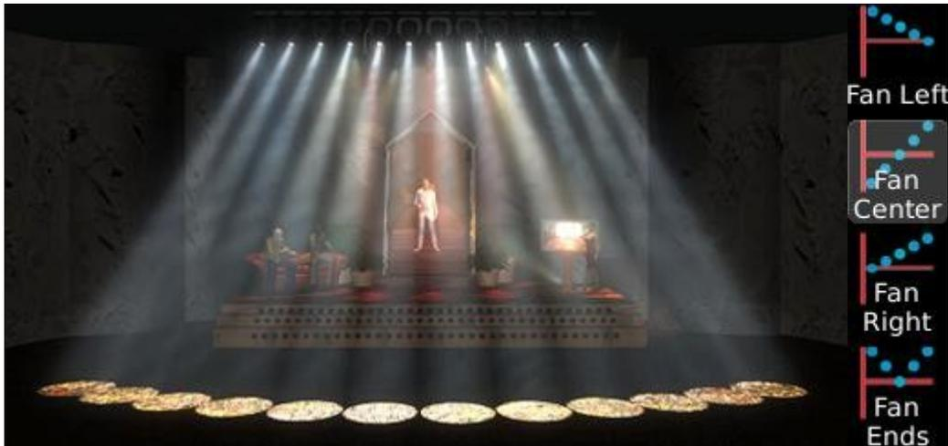
This picture shows what would happen if you selected FAN CENTER and rolled the PAN attribute. The four Fan buttons are radio buttons, i.e., only one or none can be down at any one time. Once you press one, the next time you use a Wheel, the attribute values will not be shown in their regular units, but rather a % is shown. You can roll the wheel left or right for negative or positive fanning (fan in or fan out).
