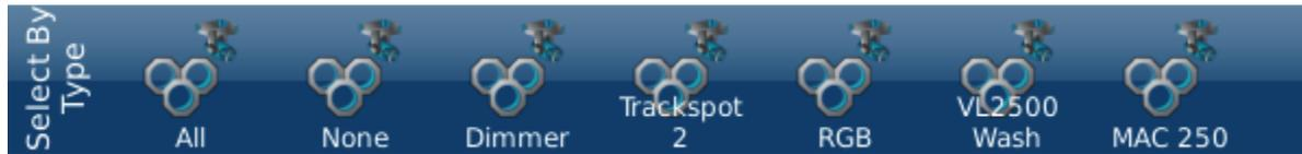
The Type tool allows quick selection such as All Lights, No Lights or by fixture types. Cognito automatically creates Standard groups of identical lights, as the lights are patched into the Fixture Grid.
