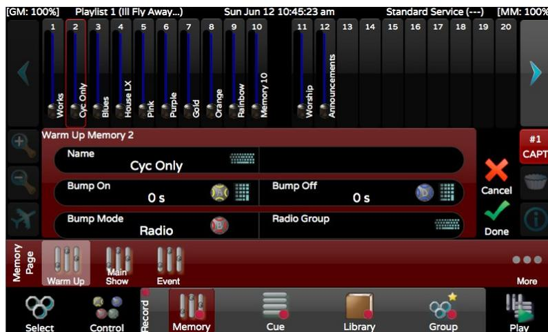
Any fader location may be chosen by touching it. The selected location is indicated by a red outline. By default, fader 1 or the next available fader is selected. Although only 20 faders are shown at one time, up to 400 memory
