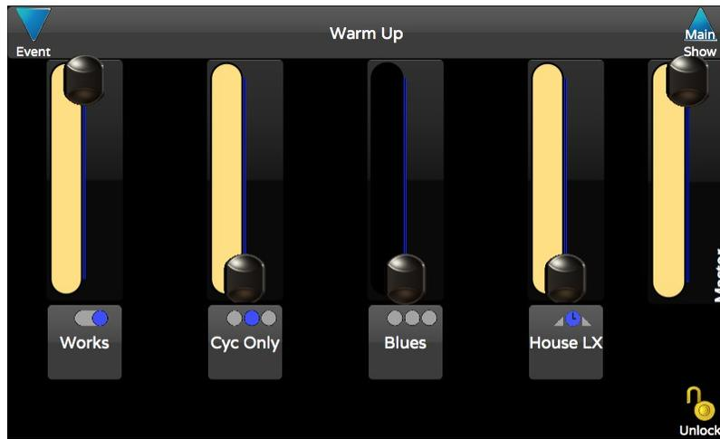
This option turns the Cognito into a virtual button/slider station. The number of Memories shown, the Memory Page associated with those buttons and password protection may be set. Once the parameters are set, touch the Lock icon to enter station mode.
