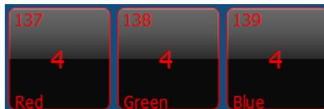
The small number at the top of each cell is the DMX slot number. The large number in the middle of each cell is the number of the light patched to that slot, and at the bottom of each cell is a brief description of the attribute that
