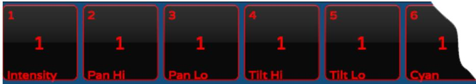
The larger number in the middle of each cell is the Light's number. At the bottom of the cell is the attribute controlled by that slot, such as intensity, color, pan,
