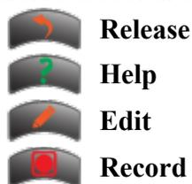
The buttons are backlit when a given function is available, and flash when that function has been selected.
