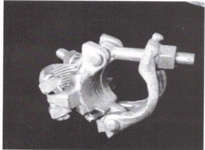
Right angle #1. Ultimate load of 14,580 lbs
