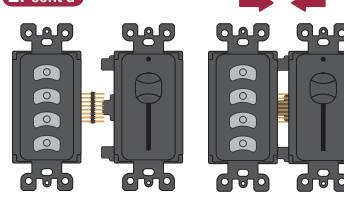
Verify proper contact by looking at the pins between the two inserts.
