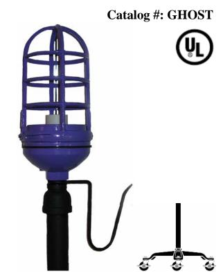
The Behind the Scenes Ghostlight comes with the protective basket and base assembly finished in Behind the Scenes Purple. The stand and locking three-wheeled base are finished in black enamel. The unit is furnished with a 15' 12/3 SJ cable with a parallel blade and ground connector; cable hook; and a medium screw-base socket. The unit is UL-Listed as a Portable Luminaire, Issue BK 09976 and is rated for a 100-Watt maximum Type A lamp.
