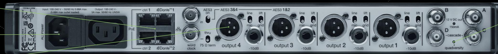
Cascade antenna ports can be switched to Quadversity inputs
