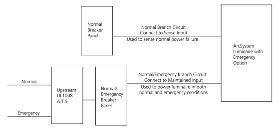
The sense input is used to detect whether normal utility power has been lost. This will force the luminaire on at 100% intensity running from the maintained supply. There is no control of the luminaire via wireless- or wired-DMX until normal utility power is restored to the sense input.
