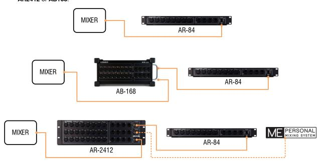
① A maximum of two dSnake remote units can be connected to each mixer's dSnake port.
