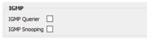
When using multicast data packets, such as streaming ACN (sACN), bandwidth efficiency may be improved by using IGMP (Internet group management protocol) to enable multicast filtering.
