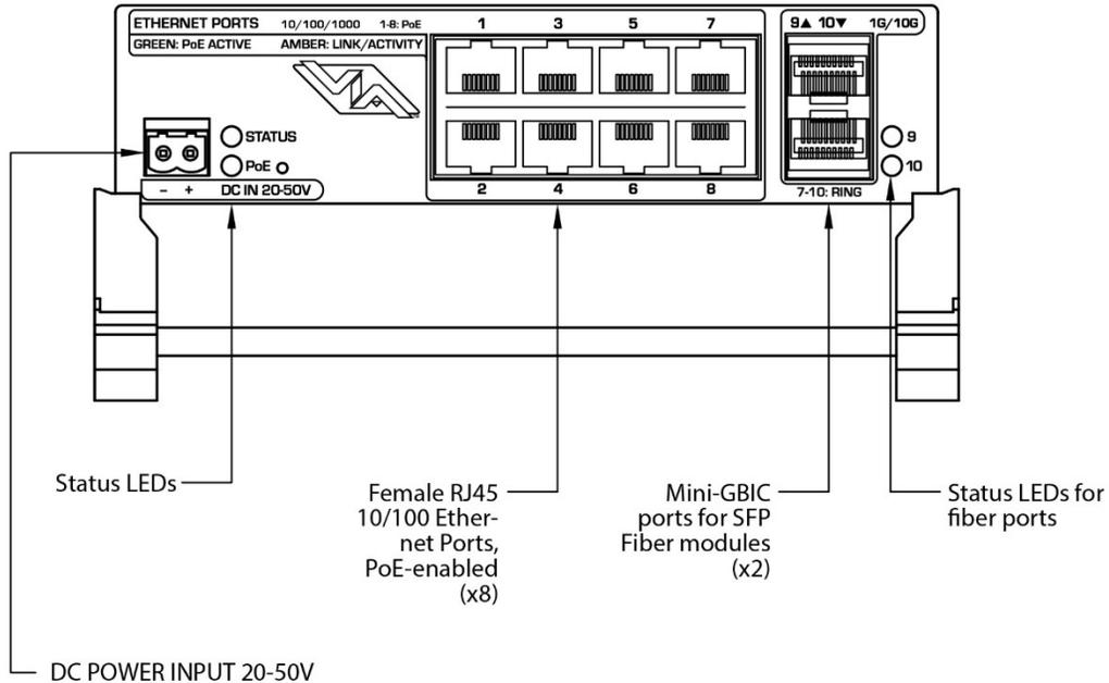
The user must provide an SFP (small-form pluggable) or SFP+ fiber adaptor to allow connection of the mini-GBIC ports to fiber optic networks. Use Pathway part number 6798 or 6799, or see Appendix 1 for recommendations on SFP adaptor selection.
