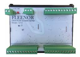
The 1212 is an economical bi-directional DMX512/RDM isolated splitter. These splitters have fully isolated inputs. The twelve outputs are separately driven, but are not isolated from one another.
