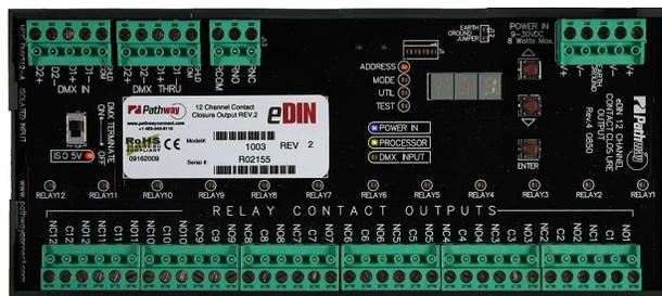
they need two connections each, as the switches provide no voltage or current on their own. One connection is to the supply and one to the load. Each relay has three sets of contacts; normally open (NO), normally closed (NC) and common (C). Generally, the normally open contacts are used, providing an open switch that closes when the relay is energized. Normally closed contacts operate in the opposite manner, providing a closed switch that opens when the relay is energized.
